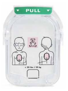
The system senses when the special Infant/Child SMART Pads cartridge is installed, and automatically adjusts CPR instructions and shock energy to a level more appropriate for infants and children under 25 kg or 55 lbs. or 0-8 years old.
